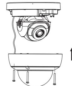
**Press Reset button for about 10s when the camera is powering on or rebooting to restore the default settings, including the user name, password, IP address, port No., etc.**
