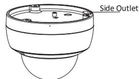
2.3. Route the cables and fix the mounting base on the ceiling with three screws.
